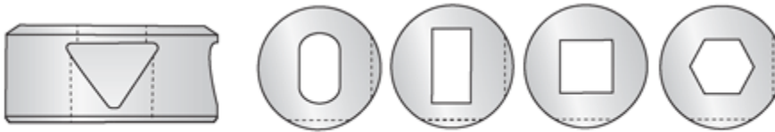
Orientation of standard whistle notches relative to shapes
